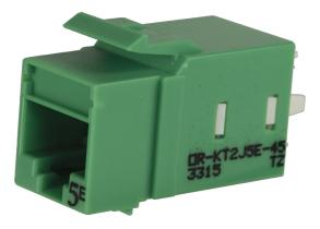
Category 5e Keystone jack, 8-position, 180 degree exit, icon compatible, T568A/B wiring, Green , individually packaged.Keystone, KT2J jacks and modules feature New installer friendly lacing cap termination with free termination tool in every carton. The keystone footprint allows flexibility in installation scheduling because its rear insertion into the faceplate allows the technician to complete the termination before and during the construction process.
