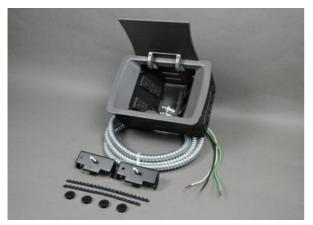
Field-wired with gray, flush cover with decorative recess. Unit comes with two 20A gasketed prewired receptacles with a 3/8" (9.5mm) diameter 6' (1.83m) flexible whip. Includes adapter for Ortronics Series II and TracJack inserts. Communication modules sold separately.
