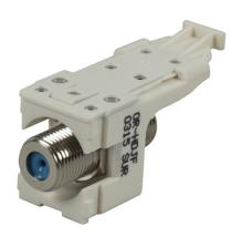
High density jack module provides a single F-connector coupler F/F with under .2dB of insertion loss at 2GHz (1/3 the loss of standard models). HDJ is a versatile single jack solution in a easy mount rear load footprint which allows a choice of up to six jacks/connectors to fit in a single gang plate, also mountable in HDJ panels.
