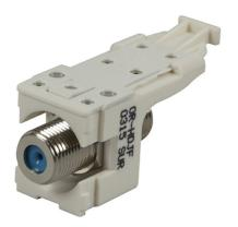
High density jack module provides a single F-connector coupler F/F with under .2dB of insertion loss at 2GHz (1/3 the loss of standard models). HDJ is a versatile single jack solution in a easy mount rear load footprint which allows a choice of up to six jacks/connectors to fit in a single gang plate, also mountable in HDJ panels.
