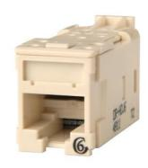
Clarity High Density Jacks (HDJ) unshielded are available in CAT5E, CAT6 and CAT6A, featuring lacing cap termination with icon slot for port ID. Jacks are sold in carton of 20, or bulk pack of 25, termination tool is included with each carton.
