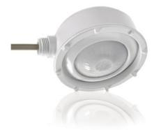
HB3x0W-Lx occupancy sensors are designed for automatic lighting control in warehouses and other medium and high bay wet location applications. They are modular and are made up of two parts, a Power Module (HB3x0W) and a Lens (HBLxW), sold separately or in prepackaged combinations. These components are designed to work as a convenient system. Different models offer a choice of coverage patterns for a range of applications.
