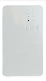
The WiFi to RFLC Bridge enables the Intuity Automation Controller to operate compatible Legrand RFLC lighting devices. Mounting to a single gang wall box and communicating via WiFi to the Intuity HA7000, the WiFi to RFLC Bridge allows control using Leg
