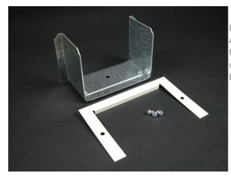
For connecting 6000 Series Raceway with surface type panel boxes. Accommodates maximum wire capacity of 6000 system. Separate Cflange fits around raceway, covering any irregularities made when cutting into box. Cut 4 3/4'' x 3 9/16'' (121mm x 90mm) hole in panel box.
