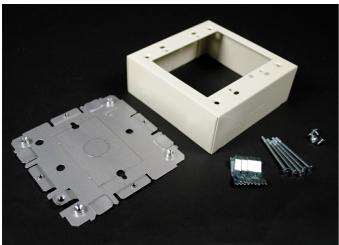
Two Gang Device Box. Cover has twistouts for 2000, 500 and 700 Series Raceways. Base has 1/2" trade size KO and rectangular KO for extension to wall box. Base has #10 threaded hole for ground connection.
