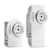
FSP-2x2 sensors provide multi-level control based on motion and/or daylight contribution. They control 0-10VDC LED drivers or dimming ballasts, as well as non-dimming ballasts and, with an FSP-Lx Lens, are rated for wet and cold locations. Line and low voltage models are available, and choice of control modes simplifies sensor configuration.
