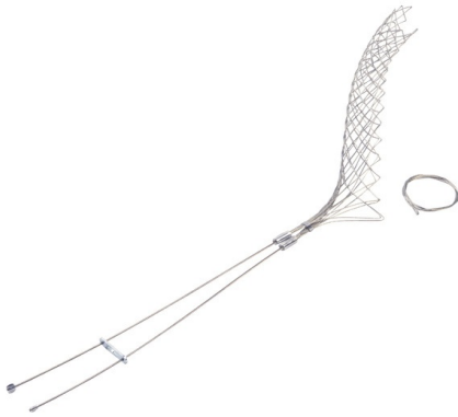
FS250LB: Standard Duty, Split Lace, Locking Bale (Universal Eye), Cable Diameter 2.50 - 2.99 inches, Bale Length 18-in, Mesh Length 24-in, Break Strength 3360 lbs.
