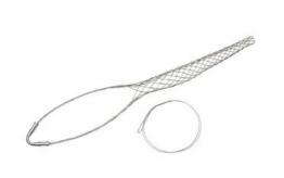
FS100U: Standard Duty, Split Lace, Single Eye, Cable Diameter 1.00 - 1.24 inches, Bale Length 9-in, Mesh Length 15-in, Break Strength 1680 lbs.
