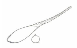
Stainless Steel, Standard-duty, Split lace, Single eye. Cable diameter - 0.750-0.990\'\', Bale length - 8\'\', Mesh length - 14\'\', Break strength - 1,320 lbs.
