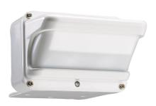
The FS-705 Wide Angle PIR Occupancy Sensor controls lighting based on occupancy utilizing passive infrared (PIR) technology. The sensor provides 180 degree coverage and is designed for locations that require wide angle occupancy detection, such as refrigerator and freezer cases, vending machines and aisleway displays.
