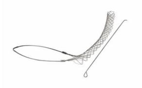
Stainless Steel, Standard duty, Split rod, Single eye. Cable diameter - 2.000-2.490\'\', Bale length - 16\'\', Mesh length - 22\'\', Break strength - 3,760 lbs.
