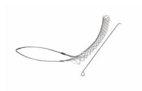
FR200U: Standard Duty, Split Rod, Single Eye, Cable Diameter 2.00 - 2.49 inches, Bale Length 16-in, Mesh Length 22-in, Break Strength 3760 lbs.
