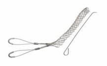
FR125UU: Standard Duty, Split Rod, Double-Eye, Cable Diameter 1.25 - 1.49 inches, Bale Length 5-in, Mesh Length 16-in, Break Strength 1680 lbs.
