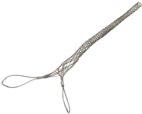
FCHL350UU: Heavy-Duty, Closed Mesh, Double-Eye, Cable Diameter 3.50 - 3.99 inches, Bale Length 10-in, Mesh Length 45-in, Break Strength 13120 lbs.
