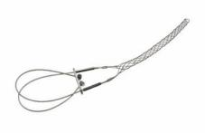
FC250LB: Standard Duty, Closed Mesh, Locking Bale (Universal Eye), Cable Diameter 2.50 - 2.99 inches, Bale Length 18-in, Mesh Length 24-in, Break Strength 3360 lbs.
