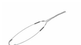
FC22: Bus Drop, Closed Mesh, Single Eye, Cable Diameter 0.22 - 0.32 inches, Bale Length 9-in, Mesh Length 3.5-in, Break Strength 1100 lbs.
