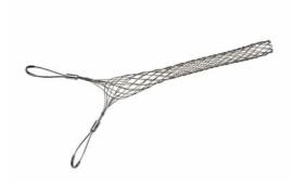
FC200UU: Standard Duty, Closed Mesh, Double -Eye Grip, Cable Diameter 2.00 - 2.49 inches, Bale Length 6-in, Mesh Length 22-in, Break Strength 3360 lbs.
