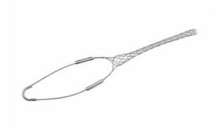
Stainless Steel, Standard-duty, Closed mesh, Single eye grips. Cable Diameter -1.750-1.990\'\', Bale length - 14\'\', Mesh length - 20\'\', Break strength - 2,640
