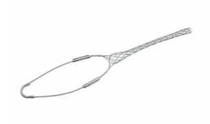
Stainless Steel, Standard-duty, Closed mesh, Single eye grips. Cable Diameter -1.500-1.740\'\', Bale length - 12\'\', Mesh length - 18\'\', 1,680 lbs.
