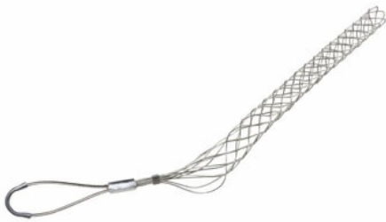
FC125OF: Standard Duty, Closed Mesh, Offset Eye Grips, Cable Diameter 1.25 - 1.49 inches, Bale Length 5-in, Mesh Length 16-in, Break Strength 1680 lbs.
