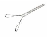
FC100UU: Standard Duty, Closed Mesh, Double -Eye Grip, Cable Diameter 1.00 - 1.24 inches, Bale Length 5-in, Mesh Length 15-in, Break Strength 1920 lbs.
