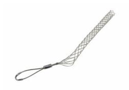
FC1000F: Standard Duty, Closed Mesh, Offset Eye Grips, Cable Diameter 1.00 - 1.24 inches, Bale Length 5-in, Mesh Length 15-in, Break Strength 1680 lbs.
