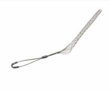
FC0750F: Standard Duty, Closed Mesh, Offset Eye Grips, Cable Diameter 0.75 - 0.99 inches, Bale Length 4-in, Mesh Length 14-in, Break Strength 960 lbs.
