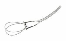
FC075LB: Standard Duty, Closed Mesh, Locking Bale (Universal Eye), Cable Diameter 0.75 - 0.99 inches, Bale Length 18-in, Mesh Length 14-in, Break Strength 1320 lbs.
