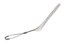
FC0620F: Standard Duty, Closed Mesh, Offset Eye Grips, Cable Diameter 0.62 - 0.74 inches, Bale Length 4-in, Mesh Length 11-in, Break Strength 960 lbs.
