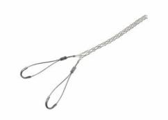
FC050UU: Standard Duty, Closed Mesh, Double -Eye Grip, Cable Diameter 0.50 - 0.61 inches, Bale Length 4-in, Mesh Length 11-in, Break Strength 770 lbs.
