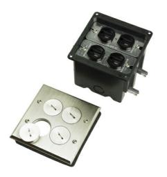
Tamper-Resistant Floor Box Assembly, Two #8 duplex openings, Four threaded screw plugs. Includes two 3232 15A, 125A tamperresistant duplex receptacles. Nickel. For detailed Tamper-Resistant receptacle information, visit our Tamper-Resistant Receptacles page.
