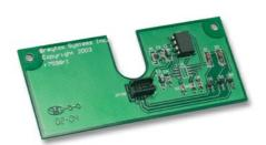
The three-note door chime attaches to the intercom module. It sounds a different chime at up to three door units when the door so button is pressed.
