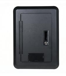
Decorative wall box cover designed to fit onto the 4-gang hinged wall box (EHWB4). Cover comes complete with a hinge that allows the cover to open a full 180 degrees, an integrated handle with lock and key set, and an egress door that allows the cables to exit the box flush against the wall. The cover is offered in two powder-coated finishes white: EHWBC4-WH or black EHWBC4-BK.
