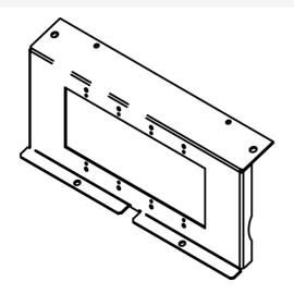
Holds a standard 4-gang device plate. Device plate dimensions: 8 1/8" x 4 1/4" (206mm x 116mm).
