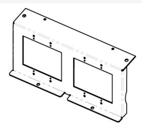
Equipped with two (2) 2-gang standard size device openings for a standard 2-gang (4 9/16'' x 4 1/2'' (116mm x 114mm)). Ideal for 2-gang A/V devices such as Crestron 2-gang digital media devices. Device plates and devices supplied by others.
