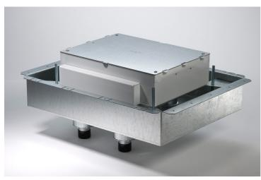
6-Gang Fire Classified Floor Box. Pre-assembled installation ready Floor Box has been designed to be installed in above grade concrete floors while maintaining the fire classification of the floor. This box is classified to be used in 1-, 11/2-, 2-, or 3-hour fire rated floors. Designed to accept standard size wall plates. Box comes complete with all components needed for initial installation.
