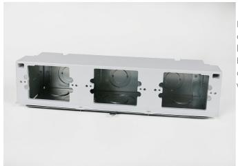
Bank of three (3) compartments that accept power, communications and audio/video devices. Accepts standard size (2 3/4" x 4 1/2" (70mm x 114mm)) device plates. Includes device bracket, back plate, three (3) knockout plates (3/4"/1 1/4" concentric), two (2) end caps and one (1) divider. NOTE: Module will fit on either side of the floor box.
