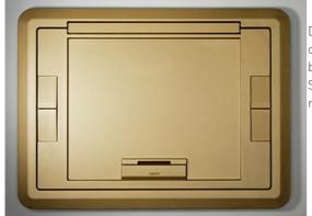
Die cast aluminum cover assembly designed to be used on top of the floor covering. Available in the following powder coated finishes: black (BK), gray (GY), brass (BS), nickel (NK) and bronze (BZ). For use on Evolution Series 6-, 8- and 10-gang floor boxes (EFB6, EFB8 and EFB10). NOTE: Depth of recess area in plate is 1/4" (6.35mm).
