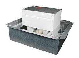
Pre-assembled installation ready floor box has been designed to be installed in above grade (second floors and above) concrete floors while maintaining the fire classification of the floor. This box is classified to be used in the 2-hour fire rated floors. Designed to accept standard size wall plates. Box comes complete with all components needed for initial installation.
