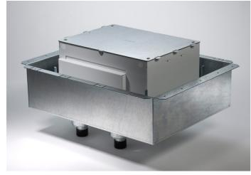
10-Gang Fire Classified Floor Box Pre-assembled installation ready Floor Box has been designed to be installed in above grade concrete floors while maintaining the fire classification of the floor. This box is classified to be used in 1-, 1 1/2-, 2-, or 3-hour fire rated floors. Designed to accept standard size wall plates. Box comes complete with all components needed for initial installation.
