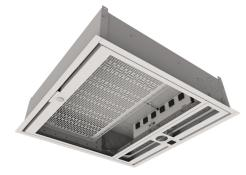
Fully finished enclosure designed to manage and store A/V equipment in an air handling plenum space above a NO or hard ceiling. These boxes are also equipped with the <u>RackLink system</u>, by <u>Middle Atlantic Products</u>. The box also has a built in projector mount that utilizes a 1 1/2" standard NFS fitting and is rated to support a load up to 50 lbs. The projector mount can move laterally and be positioned anywhere along the track.
