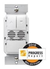
The DW-311 dual technology dimming wall switch sensor can turn lights OFF and ON based on occupancy and allow the user to increase or decrease the lighting level. It combines the benefits of passive infrared (PIR) and ultrasonic occupancy detection technologies and works with 0-10 VDC dimming drivers and ballasts to control lighting loads including LEDs.
