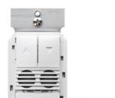
The DW-311 dual technology dimming wall switch sensor can turn lights OFF and ON based on occupancy and allow the user to increase or decrease the lighting level. It combines the benefits of passive infrared (PIR) and ultrasonic occupancy detection technologies and works with 0-10 VDC dimming drivers and ballasts to control lighting loads including LEDs.
