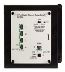
This versatile triple-speed Ethernet interface can operate as either a 4-port Gigabit Broadband Router or a 5-port Gigabit Switch, selectable with the flip of a switch. In Router mode, it so capable of up-linking with virtually any ADSL or Cable modem,
