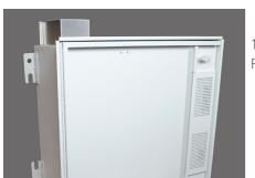
12" deep telecommunications enclosure for 2' x 2' drop ceiling tile. One removable 7 RMU bracket for 19" patch panels and equipment. Includes junction box and fan.
