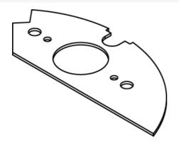
The CRFB4 has four compartments that accept different device plates. This Device Plate is for Plate location 2, accepts most 15A and 20A straight blade receptacles and 15A turnlok receptacles. NOTE: Standard size for device plates for Plate Location 2 is 5.7/32" (132mm) x 2.3/4" (62mm).
