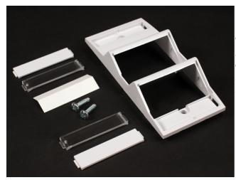
For use with multi-channel raceway device brackets and WallSource device mounting brackets. Angled exit provides additional mounting depth required for audio/visual connections as well as ensuring the required bend radius for UTP and fiber optic cabling. Holds two CM2 Series modules or two CM2 Series modules or two 2A inserts. Fits 5507 Series Faceplate opening.
