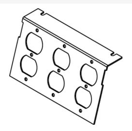
Three (3) duplex KOs for 106 communication style adapter. Fits both AC8850 and AC8105 Boxes. NOTE: AC8850 is a single-service box. Power plates cannot be used in conjunction with communication plates.
