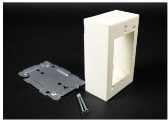
Single Gang Device Box. Cover has twistouts for 2000, 500 and 700 Series Raceways. Base has 1/2'' trade size KO and rectangular KO for extension to wall box. Base has #10 threaded hole for ground connection.
