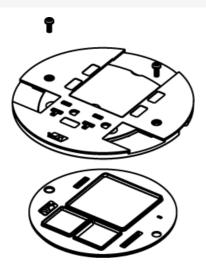
Nonmetallic slide holder assembly. Available in gray (GY), black (BK), ivory (VY), aluminum colored (AL) and brass colored (BS). NOTE: Assembled with scrub water gasket. For use on tile or carpet floors. AV3 Series Poke-Thru Devices require a 4" (102mm) diameter hole. Not designed to work with bare concrete or terrazzo. Floor covering thickness 1/8" minimum.
