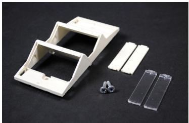
For use with multi-channel raceway device brackets and WallSource device mounting brackets. Angled exit provides additional mounting depth required for A/V connections as well as ensuring the required bend radius for UTP and fiber optic cabling. Holds two Ortronics Series II modules. Fits 5507 Series Faceplate opening. Fits 5507 Series Faceplate opening.
